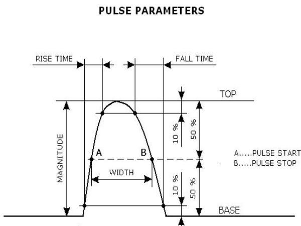
Fig. 2. A graphic presentation of the pulse parameters and their geometric sense
