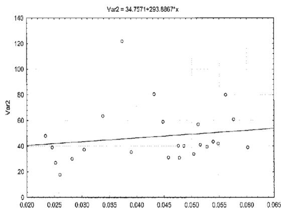
**Fig. 7.** Barley ALRAIHAN, undamaged kernels with relative humidity 0 %. The figure shows the relation between the with of impact records (vertical axis – in  $\mu$ s) and the mass of kernels (horizontal axis - in grams). The graph on the right in Figure 7 and 8 shows the borders for 95 % probability.
